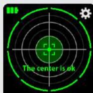
When the eccentricity is adjusted below the adjustment limit, the display switches to "The center is ok".
