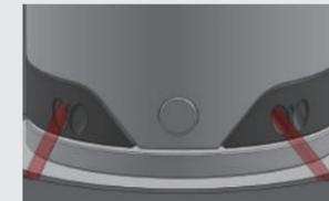
Detects end group position changes using two infrared LEDs and two linear image sensors.
