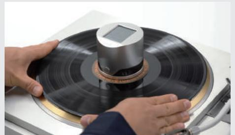
Press the record board so that the cross mark (center of rotation) is in the absolute center position.
